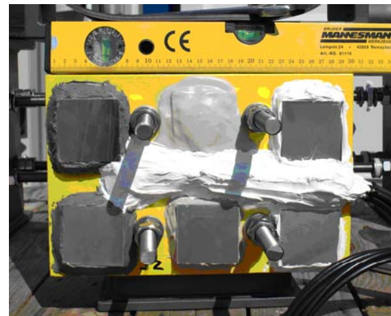
Fig. 2 Test coupon with online monitoring
